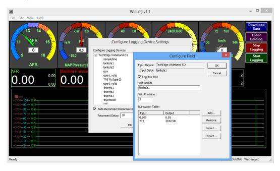
**Wideband** – load the AFR conversion of Gasoline/Petrol into the input configuration for lambda1.
